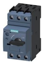
Circuit breaker size S0 for motor protection, CLASS 10 A-release 1.1...1.6 A N-release 21 A screw terminal Standard switching capacity
