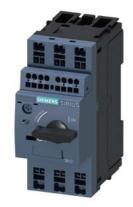
Circuit breaker size S00 for motor protection, CLASS 10 A-release 9...12 A N-release 163 A Spring-type terminal Standard switching capacity with transverse auxiliary switches 1 NO+1 NC
