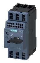
Circuit breaker size S00 for motor protection, CLASS 10 A-release 7...10 A N release 130 A Spring-type terminal Standard switching capacity with transverse auxiliary switches 1 NO+1 NC
