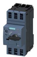
Circuit breaker size S00 for motor protection, CLASS 10 A-release 7...10 A N release 130 A Spring-type terminal Standard switching capacity
