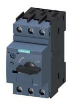
Circuit breaker size S00 for motor protection, CLASS 10 A-release 7...10 A N release 130 A screw terminal Standard switching capacity
