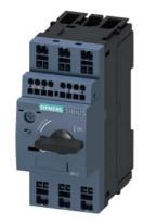
Circuit breaker size S00 for motor protection, CLASS 10 A-release 5.5...8 A N-release 104 A Spring-type terminal Standard switching capacity with transverse auxiliary switches 1 NO+1 NC
