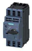
Circuit breaker size S00 for motor protection, CLASS 10 A-release 3.5...5 A N release 65 A Spring-type terminal Standard switching capacity with transverse auxiliary switches 1 NO+1 NC
