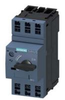
Circuit breaker size S00 for motor protection, CLASS 10 A-release 3.5...5 A N release 65 A Spring-type terminal Standard switching capacity
