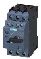
Circuit breaker size S00 for motor protection, CLASS 10 A-release 2.2...3.2 A N release 42 A screw terminal Standard switching capacity with transverse auxiliary switches 1 NO+1 NC  $\,$
