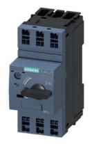
Circuit breaker size S00 for motor protection, CLASS 10 A-release 1.4...2 A N-release 26 A Spring-type terminal Standard switching capacity
