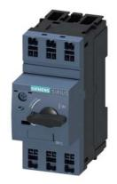
Circuit breaker size S00 for motor protection, CLASS 10 A-release 0.7...1 A N-release 13 A Spring-type terminal Standard switching capacity
