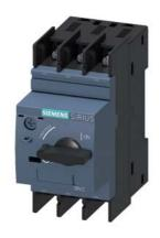
Circuit breaker size S00 for motor protection, CLASS 10 A-release 0.35...0.5 A N-release 6.5 A ring cable lug connection Standard switching capacity
