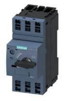
Circuit breaker size S00 for motor protection, CLASS 10 A-release 0.35...0.5 A N-release 6.5 A Spring-type terminal Standard switching capacity
