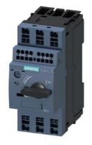
Circuit breaker size S00 for motor protection, CLASS 10 A-release 0.28...0.4 A N-release 5.2 A Spring-type terminal Standard switching capacity with transverse auxiliary switches 1 NO+1 NC  $\,$
