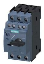
Circuit breaker size S00 for motor protection, CLASS 10 A-release 0.28...0.4 A N-release 5.2 A screw terminal Standard switching capacity with transverse auxiliary switches 1 NO+1 NC
