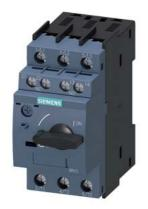
Circuit breaker size S00 for motor protection, CLASS 10 A-release 0.18...0.25 A N-release 3.3 A screw terminal Standard switching capacity with transverse auxiliary switches 1 NO+1 NC
