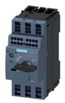
Circuit breaker size S00 for motor protection, CLASS 10 A-release 0.11...0.16 A N-release 2.1 A Spring-type terminal Standard switching capacity with transverse auxiliary switches 1 NO+1 NC
