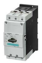
Circuit breaker size S3 A-release 36...50 A Short-circuit release 650 A Motor protection up to 100 kA,Class 20 Screw terminal Increased switching capacity !!! Phased-out product !!! Successor is SIRIUS 3RV2 Preferred successor type is >>3RV2042-4HB10<<
