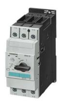
Circuit breaker size S2 for motor protection, Class 20 A-release 40...50 A Short-circuit release 650 A Screw terminal Standard switching capacity !!! Phased-out product !!! Successor is SIRIUS 3RV2 Preferred successor type is >>3RV2031-4WB10<<
