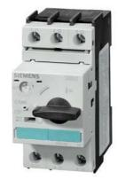
Circuit breaker size S0 for motor protection CLASS 10 A-release 11...16 A Short-circuit release 208 A Screw terminal Standard switching capacity !!! Phased-out product !!! Successor is SIRIUS 3RV2 Preferred successor type is >>3RV2021-4AA10<<
