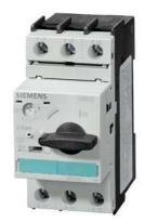
Circuit breaker size S0 for motor protection CLASS 10 A-release 0.45...0.63 A Short-circuit release 8.2 A Screw terminal Standard switching capacity !!! Phased-out product !!! Successor is SIRIUS 3RV2 Preferred successor type is >>3RV2011-0GA10<<
