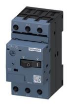
Circuit breaker size S00 for motor protection, CLASS 10 A-release 4.5...6.3 A N-release 82 A Screw terminal Standard switching capacity
