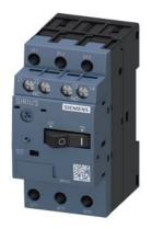
Circuit breaker size S00 for motor protection, CLASS 10 A-release 1.8...2.5 A N-release 33 A Screw terminal Standard switching capacity with transverse auxiliary switch 1 NO+1 NC
