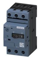
Circuit breaker size S00 for motor protection, CLASS 10 A-release 0.35...0.5 A N-release 6.5 A Screw terminal Standard switching capacity
