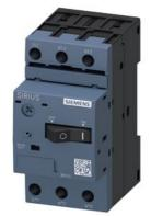
Circuit breaker size S00 for motor protection, CLASS 10 A-release 0.14...0.2 A N-release 2.6 A Screw terminal Standard switching capacity
