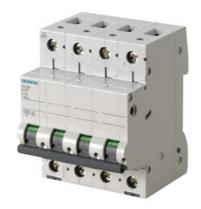
Miniature circuit breaker 400 V 6kA, 3+N-pole, C, 10 A
