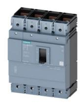
circuit breaker 3VM1 IEC frame 630 breaking capacity class N Icu=36kA @ 415V 4-pole, line protection TM210, FTFM, In=500A overload protection Ir=500A, not adjustable short-circuit protection Ii=10 x In N conductor unprotected nut keeper kit
