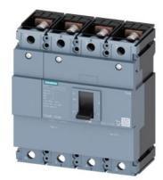
circuit breaker 3VM1 IEC frame 250 breaking capacity class S Icu=36kA @ 415V 4-pole, line protection TM210, FTFM, In=250A overload protection Ir=250A, not adjustable short-circuit protection Ii=10 x In N conductor unprotected nut keeper kit
