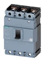
circuit breaker 3VM1 IEC frame 250 breaking capacity class S Icu=36kA @ 415V 3-pole, line protection TM210, FTFM, In=250A overload protection Ir=250A, not adjustable short-circuit protection Ii=10 x In nut keeper kit
