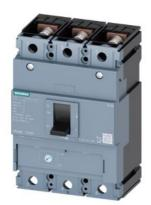
circuit breaker 3VM1 IEC frame 250 breaking capacity class N Icu=25kA @ 415V 3-pole, line protection TM220, ATFM, In=250A overload protection Ir=175A...250A short-circuit protection Ii=10 x In nut keeper kit
