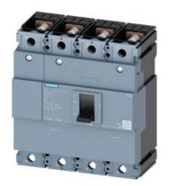
circuit breaker 3VM1 IEC frame 250 breaking capacity class N Icu=25kA @ 415V 4-pole, line protection TM210, FTFM, In=250A overload protection Ir=250A, not adjustable short-circuit protection Ii=10 x In N conductor unprotected nut keeper kit
