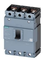
circuit breaker 3VM1 IEC frame 250 breaking capacity class N Icu=25kA @ 415V 3-pole, line protection TM210, FTFM, In=250A overload protection Ir=250A, not adjustable short-circuit protection Ii=10 x In nut keeper kit
