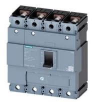
circuit breaker 3VM1 IEC frame 250 breaking capacity class S Icu=36kA @ 415V 4-pole, line protection TM220, ATFM, In=200A overload protection Ir=140A...200A short-circuit protection Ii=10 x In N conductor unprotected nut keeper kit
