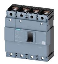
circuit breaker 3VM1 IEC frame 250 breaking capacity class S Icu=36kA @ 415V 4-pole, line protection TM210, FTFM, In=200A overload protection Ir=200A, not adjustable short-circuit protection Ii=10 x In N conductor unprotected nut keeper kit
