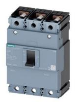
circuit breaker 3VM1 IEC frame 250 breaking capacity class S Icu=36kA @ 415V 3-pole, line protection TM210, FTFM, In=200A overload protection Ir=200A, not adjustable short-circuit protection li=10 x In nut keeper kit
