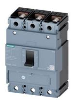
circuit breaker 3VM1 IEC frame 250 breaking capacity class N Icu=25kA @ 415V 3-pole, line protection TM220, ATFM, In=200A overload protection Ir=140A...200A short-circuit protection Ii=10 x In nut keeper kit
