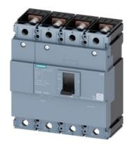
circuit breaker 3VM1 IEC frame 250 breaking capacity class N Icu=25kA @ 415V 4-pole, line protection TM210, FTFM, In=200A overload protection Ir=200A, not adjustable short-circuit protection Ii=10 x In N conductor unprotected nut keeper kit
