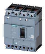
circuit breaker 3VM1 IEC frame 160 breaking capacity class S Icu=36kA @ 415V 4-pole, line protection TM220, ATFM, In=50A overload protection Ir=35A...50A short-circuit protection li=10 x In N conductor unprotected nut keeper kit
