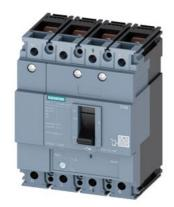
circuit breaker 3VM1 IEC frame 160 breaking capacity class S Icu=36kA @ 415V 4-pole, line protection TM220, ATFM, In=40A overload protection Ir=28A...40A short-circuit protection Ii=10 x In N conductor unprotected nut keeper kit
