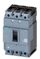
circuit breaker 3VM1 IEC frame 160 breaking capacity class N Icu=25kA @ 415V 3-pole, line protection TM220, ATFM, In=25A overload protection Ir=18A...25A short-circuit protection Ii=12.8 x In nut keeper kit
