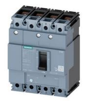
circuit breaker 3VM1 IEC frame 160 breaking capacity class S Icu=36kA @ 415V 4-pole, line protection TM220, ATFM, In=20A overload protection Ir=14A...20A short-circuit protection Ii=16 x In N conductor unprotected nut keeper kit
