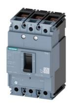
circuit breaker 3VM1 IEC frame 160 breaking capacity class N Icu=25kA @ 415V 3-pole, line protection TM220, ATFM, In=20A overload protection Ir=14A...20A short-circuit protection Ii=16 x In nut keeper kit
