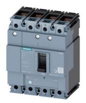
circuit breaker 3VM1 IEC frame 160 breaking capacity class S Icu=36kA @ 415V 4-pole, line protection TM220, ATFM, In=160A overload protection Ir=112A...160A short-circuit protection Ii=10 x In N conductor unprotected nut keeper kit
