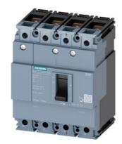
circuit breaker 3VM1 IEC frame 160 breaking capacity class S Icu=36kA @ 415V 4-pole, line protection TM210, FTFM, In=160A overload protection Ir=160A, not adjustable short-circuit protection Ii=10 x In N conductor unprotected nut keeper kit
