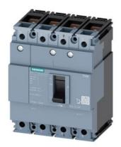
circuit breaker 3VM1 IEC frame 160 breaking capacity class S Icu=36kA @ 415V 4-pole, line protection TM210, FTFM, In=125A overload protection Ir=125A, not adjustable short-circuit protection Ii=10 x In N conductor unprotected nut keeper kit
