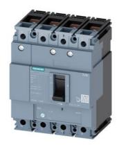
circuit breaker 3VM1 IEC frame 160 breaking capacity class S Icu=36kA @ 415V 4-pole, line protection TM220, ATFM, In=100A overload protection Ir=70A...100A short-circuit protection Ii=10 x In N conductor unprotected nut keeper kit
