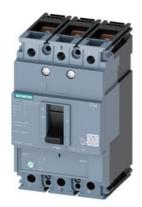
circuit breaker 3VM1 IEC frame 160 breaking capacity class N Icu=25kA @ 415V 3-pole, line protection TM220, ATFM, In=100A overload protection Ir=70A...100A short-circuit protection Ii=10 x In nut keeper kit
