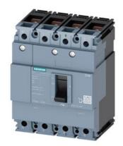
circuit breaker 3VM1 IEC frame 100 breaking capacity class S Icu=36kA @ 415V 4-pole, line protection TM210, FTFM, In=16A overload protection Ir=16A, not adjustable short-circuit protection Ii=20 x In N conductor unprotected nut keeper kit
