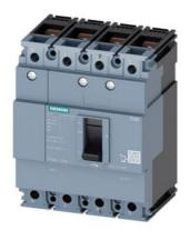
circuit breaker 3VM1 IEC frame 100 breaking capacity class S Icu=36kA @ 415V 4-pole, line protection TM210, FTFM, In=80A overload protection Ir=80A, not adjustable short-circuit protection Ii=10 x In N conductor unprotected nut keeper kit
