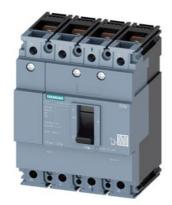
circuit breaker 3VM1 IEC frame 100 breaking capacity class N Icu=25kA @ 415V 4-pole, line protection TM210, FTFM, In=80A overload protection Ir=80A, not adjustable short-circuit protection Ii=10 x In N conductor unprotected nut keeper kit
